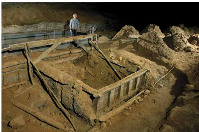
Figure 6: Remnants of saltpeper vats in Mammoth Cave, used in the early 19 th century for leaching soluble nitrates from cave sediments for the manufacture of gunpowder.
